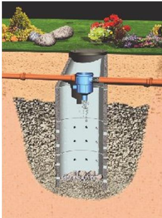
Principle of a soakaway
