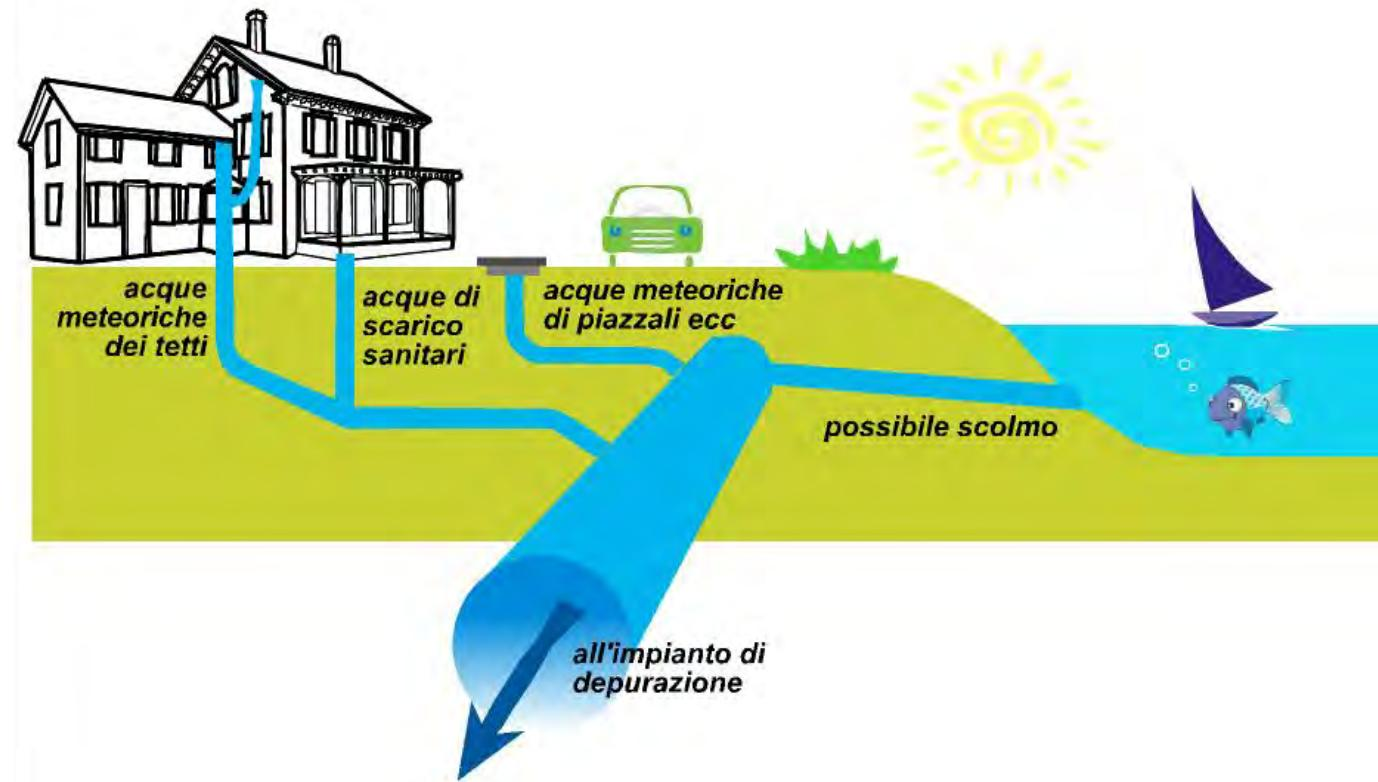
... but this solution generates side-effects whenever the sewer is connected to a treatment plant;
