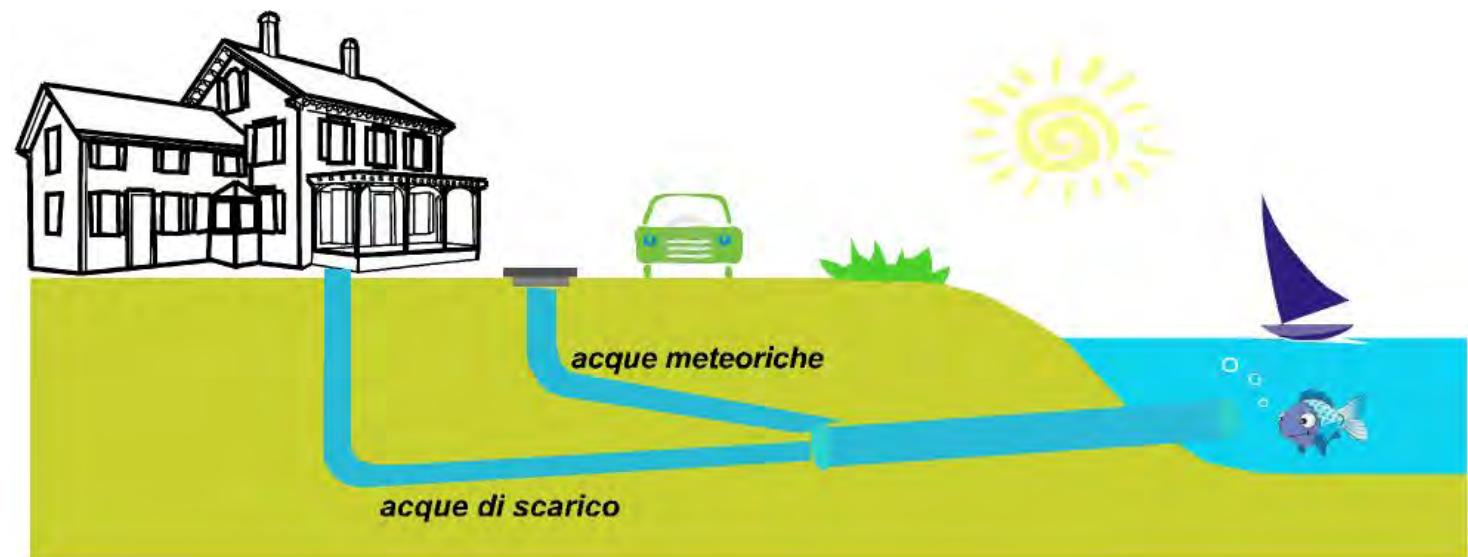
Mixed sewers represent the most adopted solution for the collection of untreated wastewater: the high flux of water permits the transport of solids and the wash-out of the sediments at every rain event.
